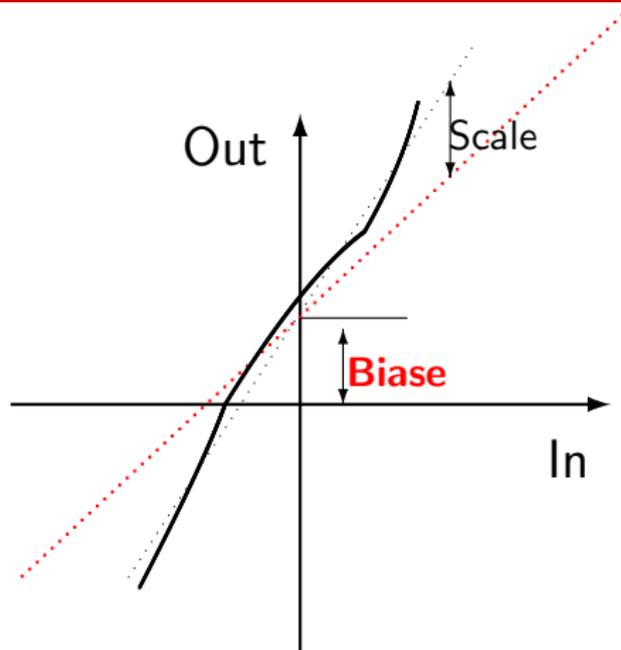
$$\tilde{f}_{ib}^b = s_{acc} \cdot \omega_{ib}^b + b_a + Noise_a$$
