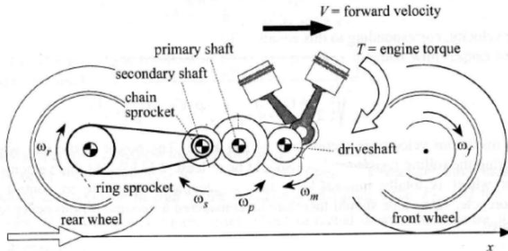
**Motor-spin** estimation may replace **wheel-spin** measurement if we know the engaged **gear state**.
